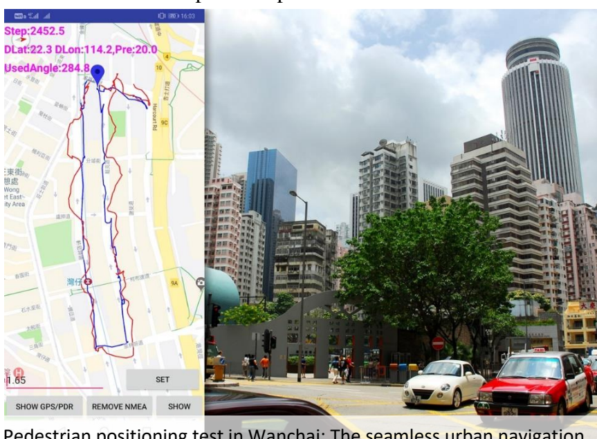
Pedestrian positioning test in Wanchai: The seamless urban navigation system (blue lines) yields far more accurate results than a smartphone (red lines).
