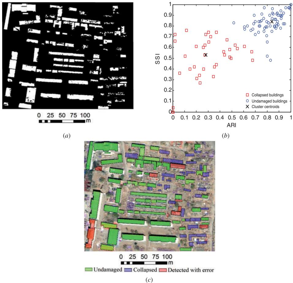
Figure 4. (a) Extracted homogeneous regions (bright parts) by improved active contour model; (b) clustering result based on SSI and ARI of buildings and (c) detected result for collapsed buildings.
