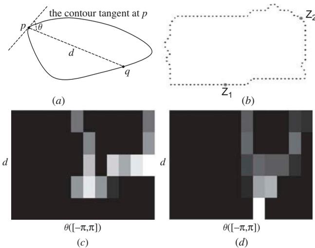
Figure 2. Establishment of shape context histograms. (a) Inner-distance and inner-angle; (b) sample points on the boundary; (c) and (d) shape context histograms of  $Z_1$  and  $Z_2$ , respectively.
