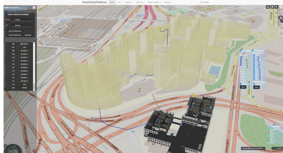
Indoor and outdoor integrated point-to-point 3D navigation (Hong Kong Polytechnic University campus)
