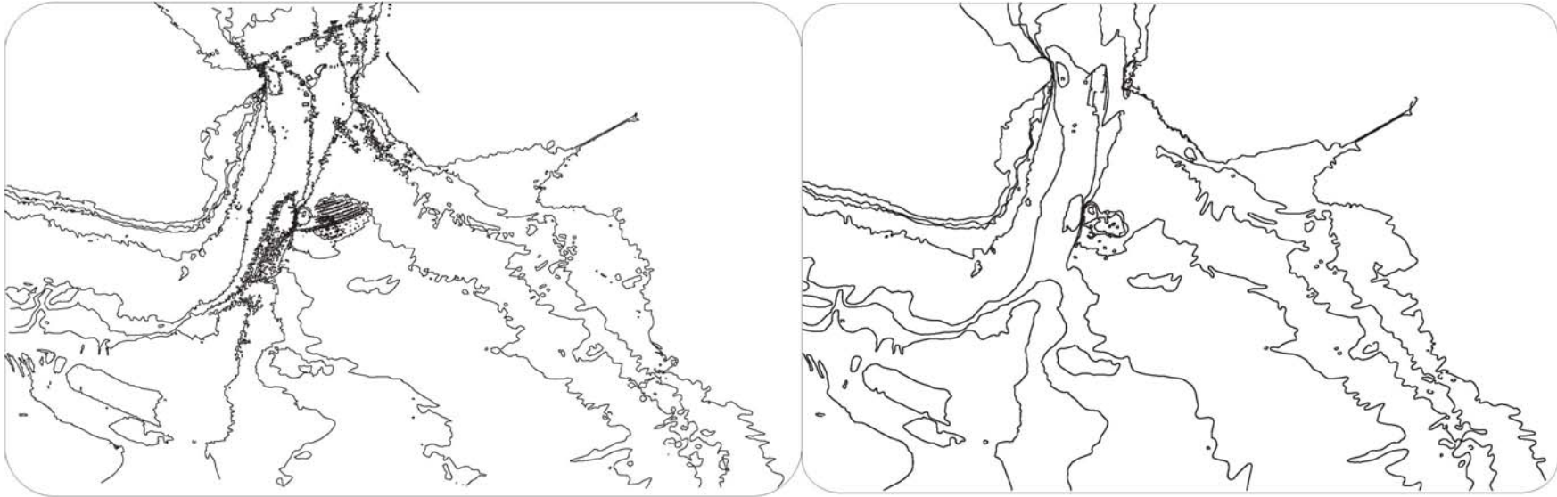
Example for generalization of nautical chart Lines before and after manual generalization
