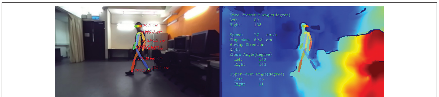
Figure 8. Visualization of the real-time photogrammetric system for human kinematics.
