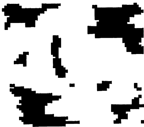
Figure 4. Result after applying erosion process to area features in Figure 1(a), some eliminated and others reduced in size.
