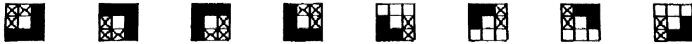
Figure 18. The series of structuring elements for convex hull formation (“x” means “don’t care”).
