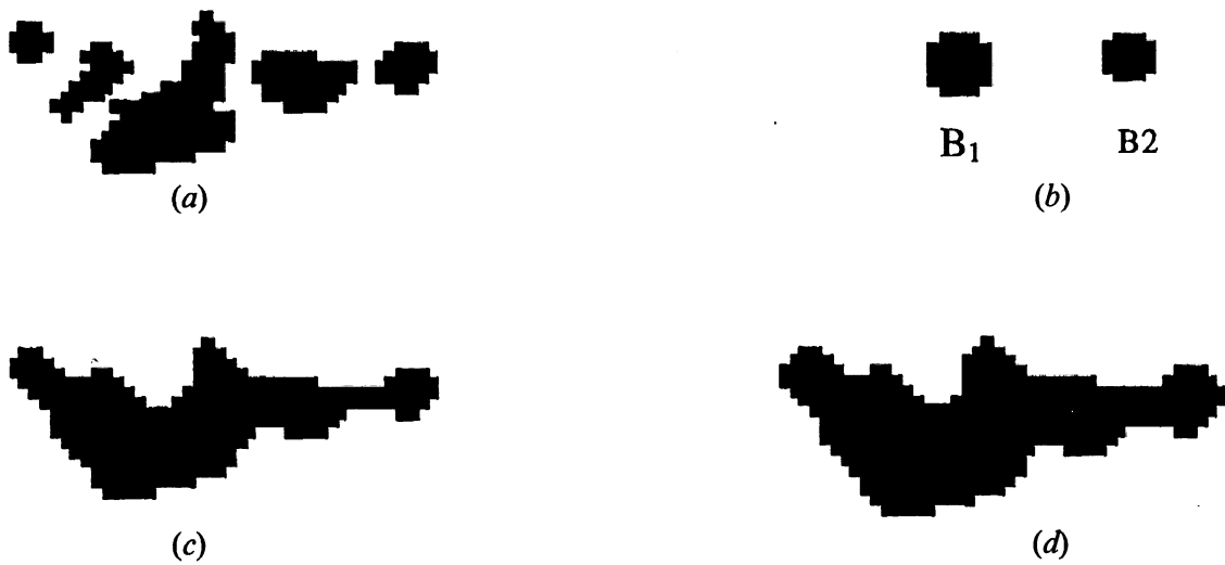
Figure 15. Combination of curved area features (II). (a) Original features A, (b) Structuring elements, (c) Areas combined C = A \cdot B_1 , (d) Combined area C = (A \oplus B_1) \otimes B_2 .
