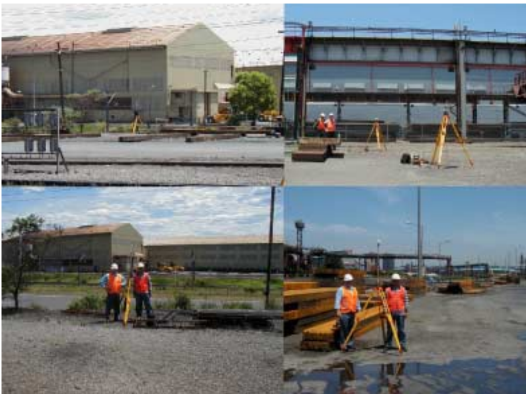
Figure 6. Location of three pseudolites (top-left, bottom-left and bottom-right) and two GPS receivers (top-right), 3 January 2001.
