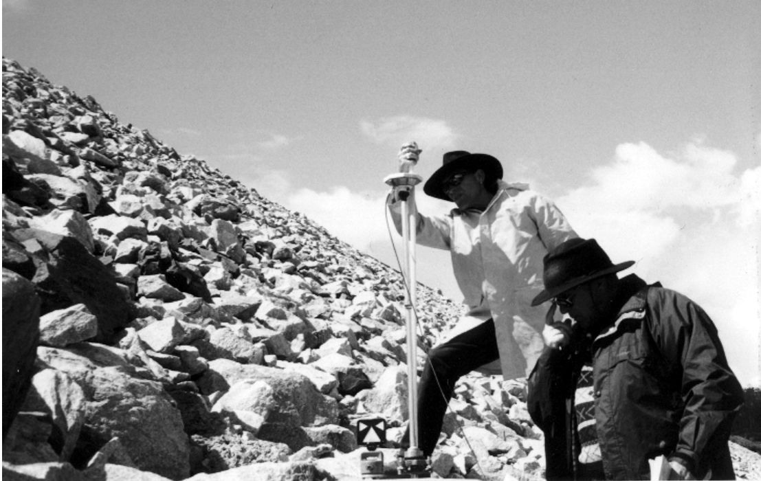
Figure 6 Antenna setup for episodic monitoring surveys
