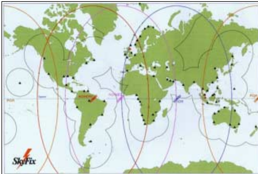
Figure 3: LandStar-DGPS network and coverage map (after Racal, 2000)
