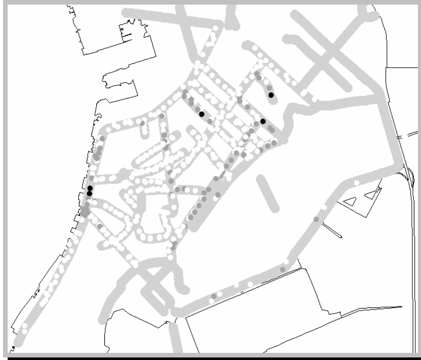
Figure 5 Modeled CO distribution (the values of 1/3, 2/3 and 3/3 of class I Chinese National Air Quality Standard requirements are displayed as white, gray and black dots respectively)
