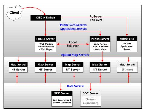
Figure 7. Web Mapping Portal public system architecture
